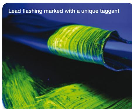
Lead flashing marked with a unique taggant
